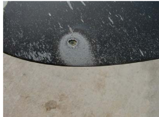
FIGURE 1-12. Lightning Strike on a Composite Surface
