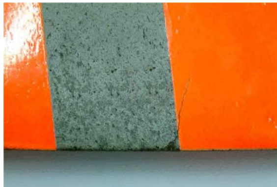
FIGURE 1-9. Blade Crack from a Nick
