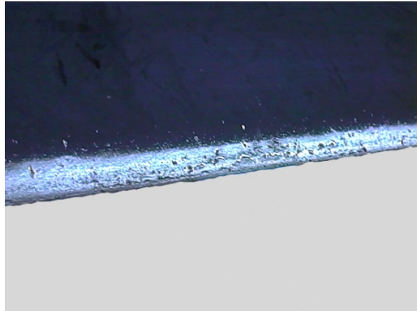
FIGURE 1-5. Exfoliation on the Blade Leading Edge
